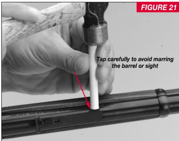
the sights set as they come from the factory (intermediate position on both elevation and windage), and then make incremental adjustments to move the sight blade and blade holder to position the group on your target. The procedures below are for the type of open sights found on many current Model 9410 shotguns.
