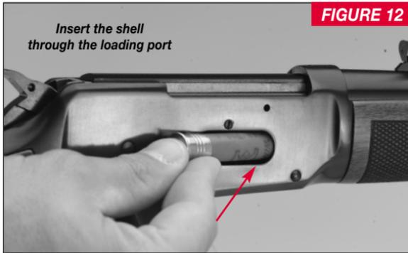
Be sure to check the shell to make sure it is a 2½" shell and not a 3" shell. If it is a 3" shell do not use it or try to chamber it in your Model 9410. Store it away separately from your gun.
