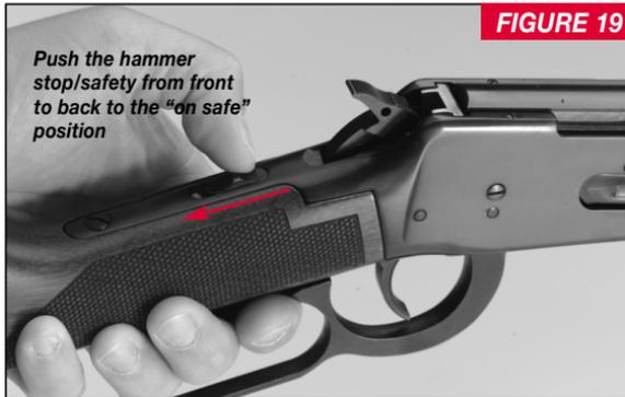
**3. WHEN THROUGH FIRING ALWAYS IMMEDIATELY PLACE THE TOP-TANG SAFETY IN THE "ON" POSITION (FIGURE 19), AND THE HAMMER IN THE SAFETY (REBOUND) POSITION (FIGURE 6).**
