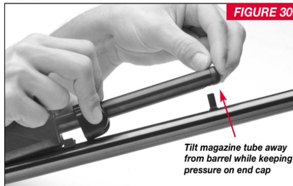
remove the magazine end cap from the magazine by tilting the magazine tube away from the barrel enough to clear the sling post mounting stud on the barrel (Figure 30). **Remember, magazine is under spring load.**
