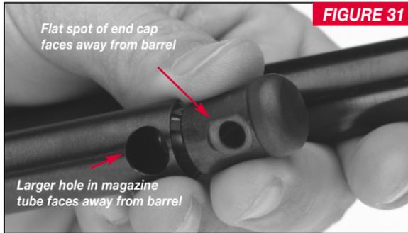
post mounting stud, note the two different sized holes in the end of the magazine tube (Figure 31). **The larger hole must face away from the barrel.**
